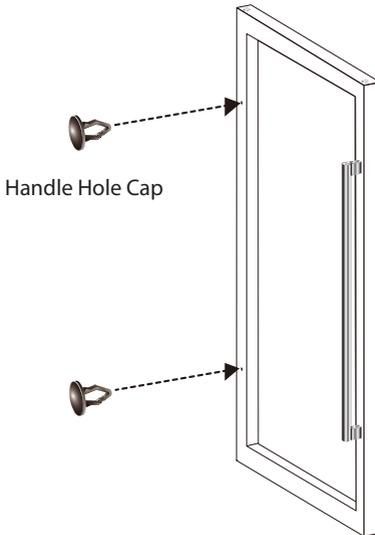
5. Remove the Handle Hole Cap (2pcs) on the right side of Door by prying it out gently with small flat screwdriver.
