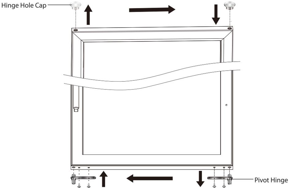
**3.** Remove the Bottom Hinge Cover by prying it off gently with small flat screwdriver. Remove the Bottom Hinge by unscrewing the Hex Head Screw (4pcs). Unscrew the Pan Head Screw (4pcs) from bottom left side. Now move the Bottom Hinge to the bottom left side and screw it tightly with the Hex Head Screws (4pcs). Move the Pan Head Screw (4pcs) to the bottom right side and screw it.
