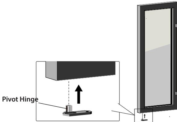
**12.** Install the door to the left hinge side by tightening the Pivot Hinge with the 2 screws.
