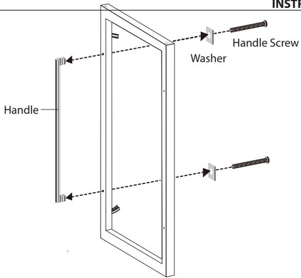
**9.** Install the Handle to the right side of the door by screwing tightly the Handle Screws (2PCS).
