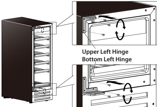
**6.** Move the Hinge Hole Cap (at the top of the door) from the left side to the right side.
