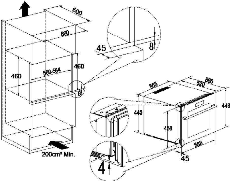
For a firmly fixing of the unit you can install an extra **Top Mounting Bar** (which is an accessory packed with the unit) onto the topside of the unit and screw it with the kitchen cabinet. See right drawing:
