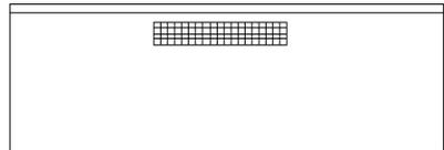
Notes: If you would like to install the wine cabinet in a place where the kitchen cabinet is entirely closed, there should be a ventilation grill on the top of the kitchen cabinet for ventilation.
