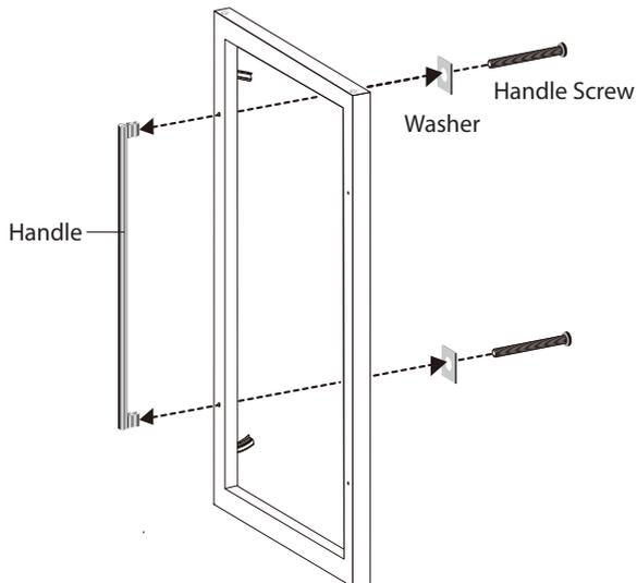
**7** Install the Handle to the right side of the door by screwing tightly the Handle Screws (2PCS).
