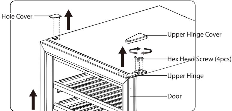
2. Move the Hinge Hole Cap (at the top of the door) from the left side to the right side. Move the Pivot Hinge (at the bottom of the door) from the right to the left side.
