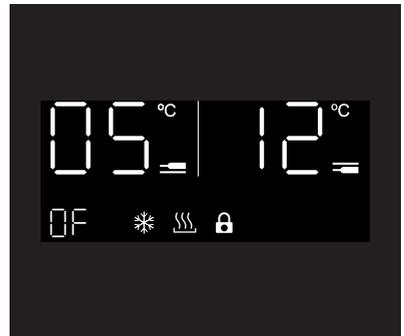
The display window can be set to the off position for a less obtrusive appearance. Your Wine Cooler will continue to run, but the Wine Coolers display window will not be visible. You can check the temperature of the Wine Cooler by pressing the **Power** button.
