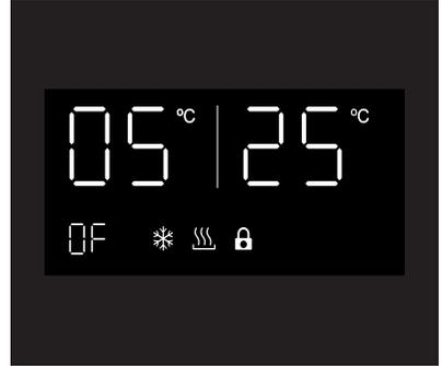
The temperature display will show the set temperature when the Wine Cooler control panel is unlocked and selected to be reset, and show the actual temperature when the control panel is locked.
