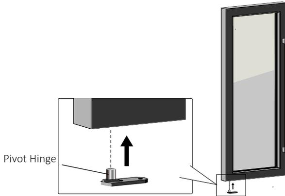
8. Install the door to the left hinge side by tightening the Pivot Hinge with the 2 screws.
