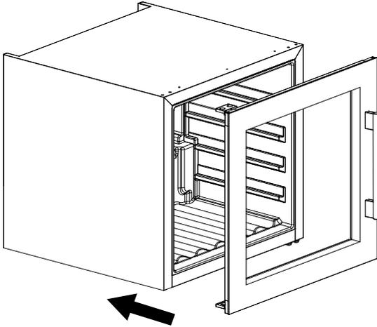
o Install the Upper Door Shaft (Left/Right) on the upper left door corner by screwing the 2 Phillips Flat Screws ( M4\*8);
