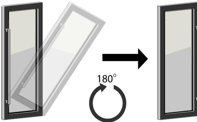
7. Insert the Pivot Hinge into the bottom hinge hole of the door.
