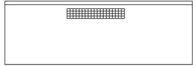
Notes: If you would like to install the wine cabinet in a place where the kitchen cabinet is entirely closed, there should be a ventilation grill on the top of the kitchen cabinet for ventilation.
